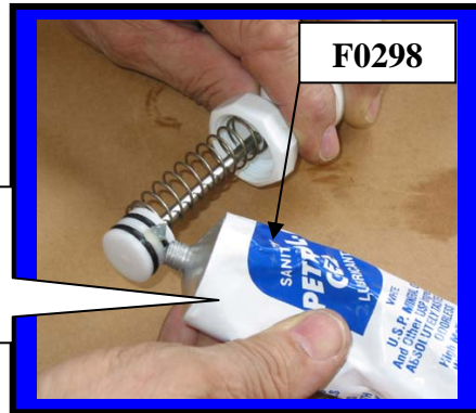
Lubricating o-rings with Petro-Gel
