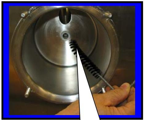
Insert short brush **F0326** into the center of the ceramic ring to remove any grease or dried product.
