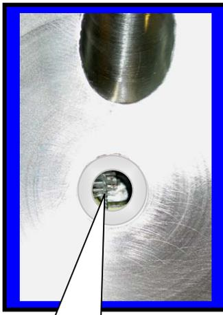
Push brush all the way in until it can be seen in the middle of the ceramic ring
