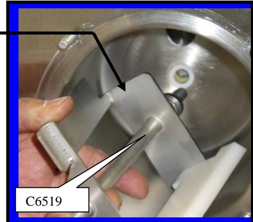
**CAUTION:** Do not strike the ceramic seal with the beater bar during installation!
