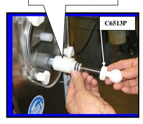
Installing **Faceplate** onto front of Machine.
