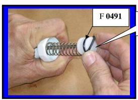
Install **O-rings** onto plunger
