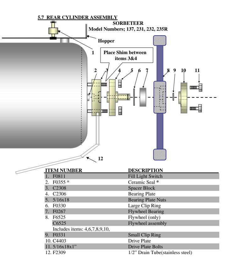
\*Note: F0355 is the part number for the <u>Spring Seal Assembly</u> which includes the ceramic seal (No.2 above)
