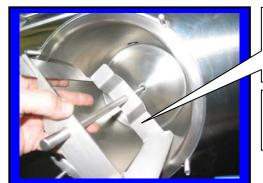
Step 7: Install large beater bar assembly C6527 into cylinder.
