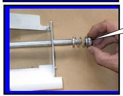
Step 5: Install spring seal **F0355**
