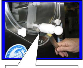
Align Faucet Assembly opening to bottom of faceplate then tighten nut
