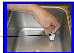
(3) Pour two gallons of cool (75°F.) water into the hopper. Clean the hopper and feed hole. Place upper switch in "faucet" position to let the machine stir for 2 minutes. Turn machine "OFF", drain and dispose of the rinse water. Repeat until water is clear.
