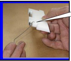
Step 1: Attach scraper blade <u>spring</u> **F6517**as shown.
