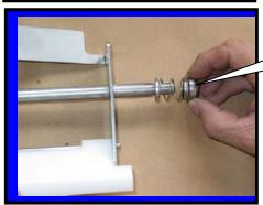
Step 5: Install spring seal **F0355**
