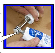
Installing Plunger assembly **C6513P** into faucet body
