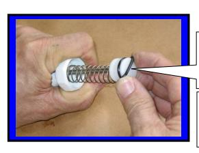
Installing o-rings onto plunger F **0491**
