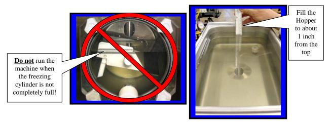
When the cylinder is full and the hopper is filled to one inch from the top, the machine is ready to run. Turn on by selecting the "right" (snowflake) position of **both** switches on the front panel.
