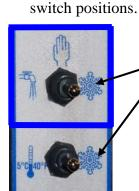
**Normal Operation** – Both switches on **snowflake.** Machine will freeze mix to provide frozen beverage as desired.
