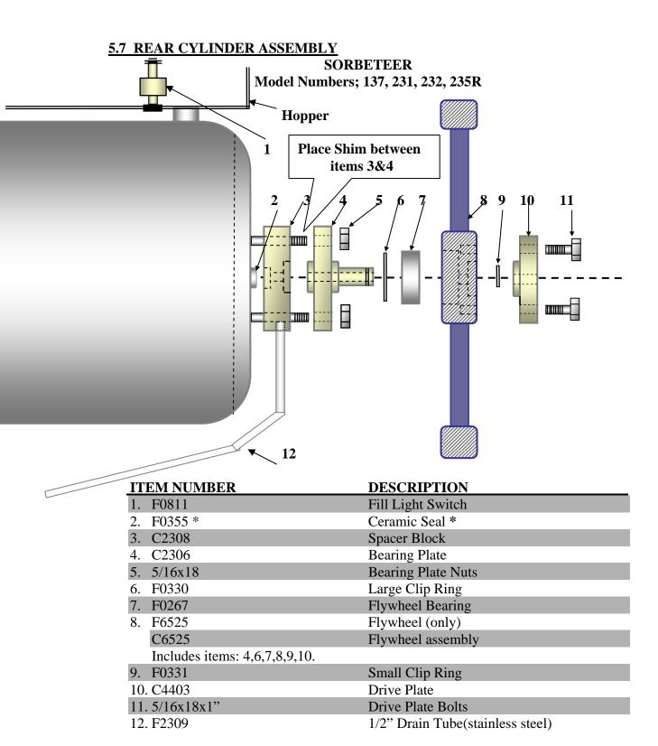
\*Note: F0355 is the part number for the <u>Spring Seal Assembly</u> which includes the ceramic seal (No.2 above)
