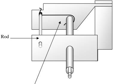
Spring position is shown without scraper blade for clarity
