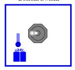
**Cooling Operation -** Machine will automatically come on whenever necessary to keep mix cooled to (5 ° C) 40 ° F. This function is used primarily for overnight storage of the mix remaining in the machine. **NOTE: Top switch** *must* be in the snowflake position.
