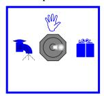
**Normal Operation -** Machine will freeze mix to provide frozen beverage. **NOTE: Bottom switch** must also be in the snowflake position. *(The faceplate must be installed for the motor to run)*
