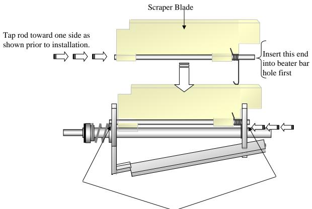
After installation tap rod until evenly spaced in beater bar as shown.
