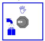
**Cleaning Operation -** The drive motor will run in the faucet position to allow a stirring action of the rinse water while cleaning. No freezing or cooling available in this position. (*The faceplate must be installed for the motor to run*)
