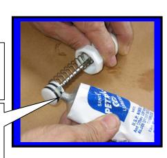
Installing Plunger assembly **C6513P** into faucet body
