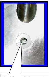
Push brush all the way in until it can be seen in the middle of the ceramic ring
