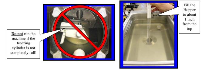
When the cylinder is full and the hopper is filled to one inch from the top, the machine is ready to run. Turn on by selecting the "right" (snowflake) position of **<u>both</u>** switches on the front panel.
