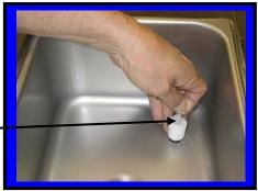
(3) Pour two gallons of cool (75°F.) water into the hopper. Clean the hopper and feed hole. Place upper switch in "faucet" position to let the machine stir for 2 minutes. Turn machine "OFF", drain and dispose of the rinse water. Repeat until water is clear.
